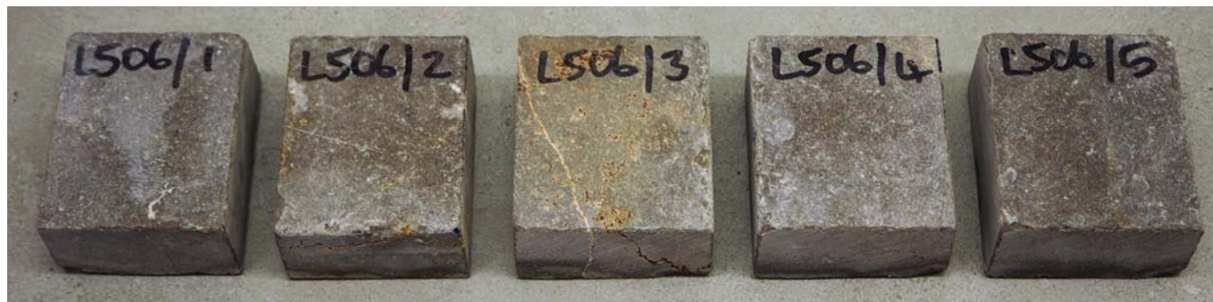
Plate 1: Appearance of Ardenne Limestone after durability testing.
